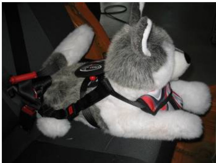
Figure 3: Dog harness with double tie-in to vehicle belt
