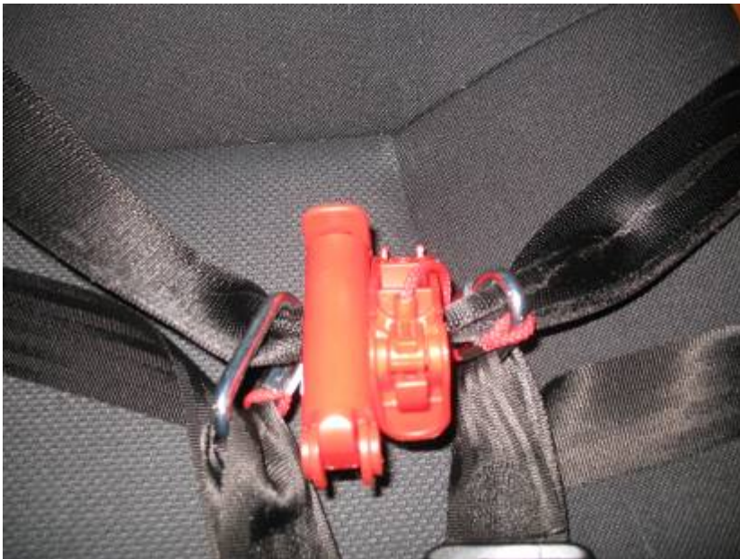
Figure 15: Under load, the clamps shift towards the centre of the lap belt creating considerable belt slack
