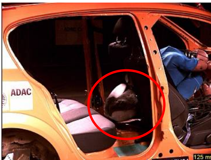
Figure 13: 125ms – the dog dummy bumps into the driver's backrests, causing extreme deformation
