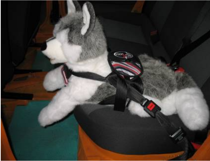
Figure 14: Carabiners and clamps are used to attach the dog harness on either side
