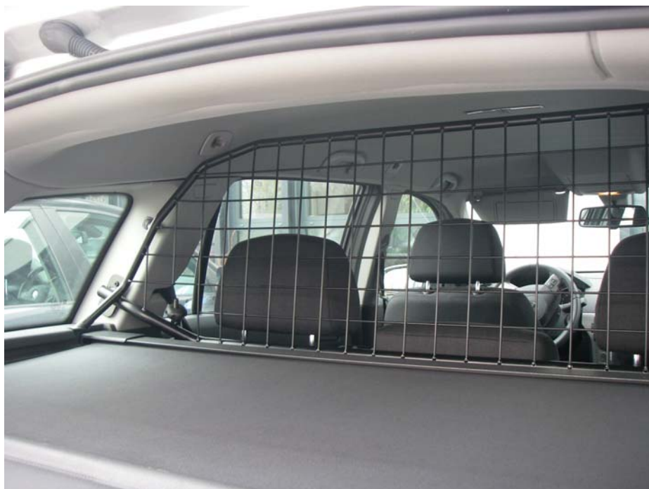
Figure 6: Partition grille for estate cars
