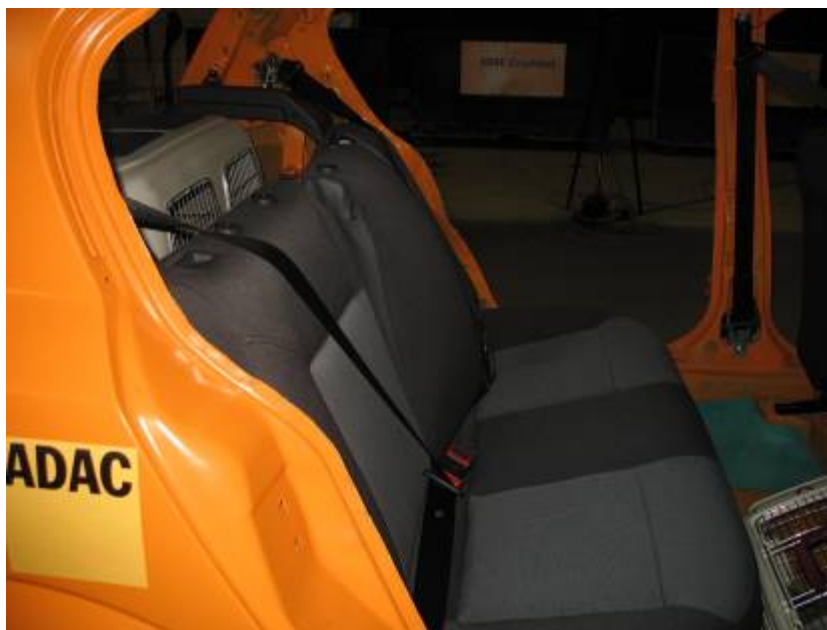
Figure 25: Post-crash deformation showing the high load on the rear backrest
