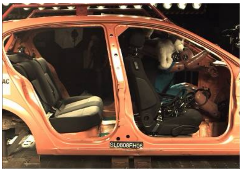
Figure 9: 150ms – the dog strongly deforms the backrests and hits the driver's head and neck
