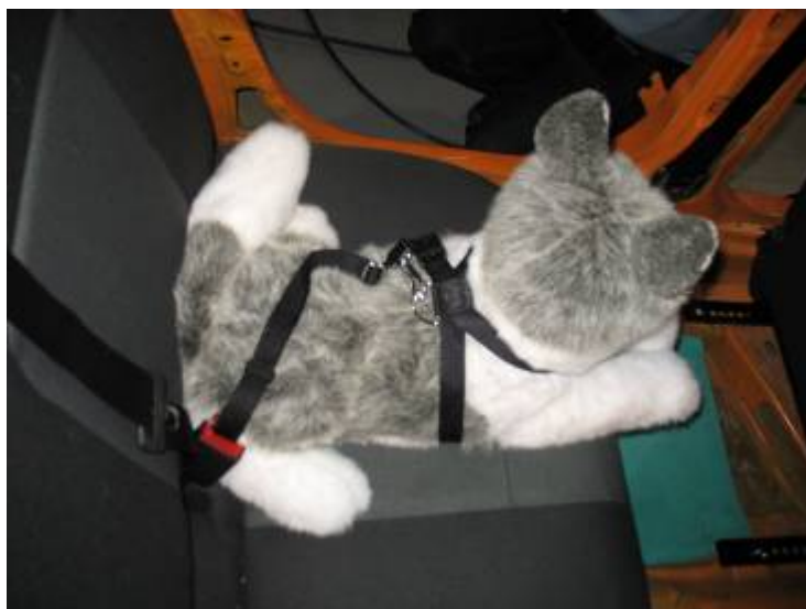
Figure 4: Dog harness with single tie-in to belt buckle
