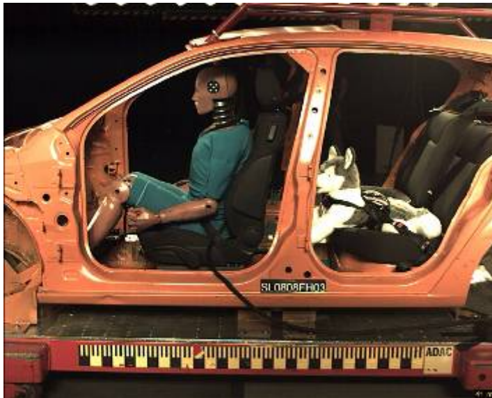
Figure 16: 0ms – the dog in its original position
