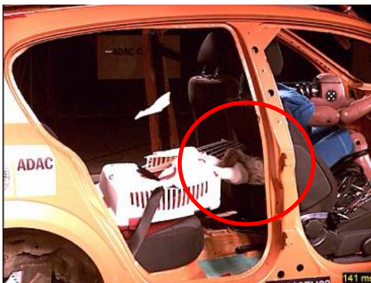
Figure 22: 140ms – the dummy flings the trap door open before hitting the front passenger backrest at almost full speed
