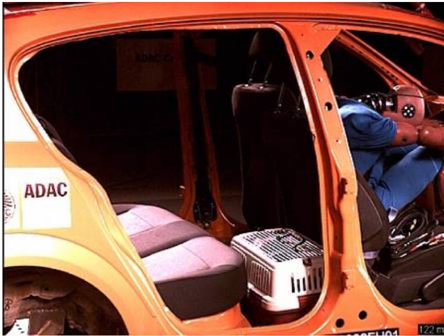
Figure 23: Good restraint of the pet carrier and even load distribution
