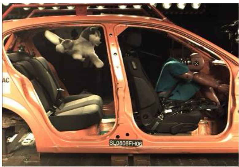
Figure 8: 50ms – the dog dummy is hurled across the cabin unrestrained
