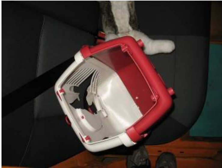
Figure 19: Pet carrier trap door torn from its hinges and belt attachment points destroyed
