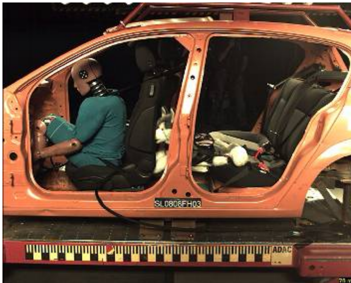
Figure 17: 75ms – upon the impact, the dog is hurled forward. The load makes the belt clamps shift towards the centre, and the seatbelt slackens
