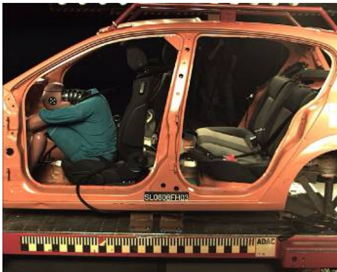
Figure 18: 100ms – the dog harness restrains the pet only after it hit and deformed the driver's backrest
