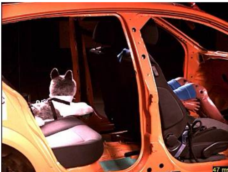
Figure 11: 0ms – the dog in its original position on the rear bench
