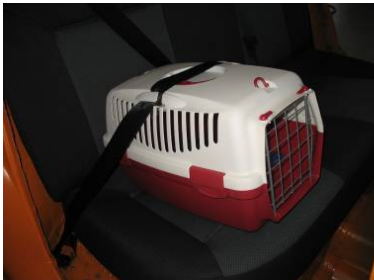
Figure 2: Small pet carrier secured on rear seat as recommended by the manufacturer
