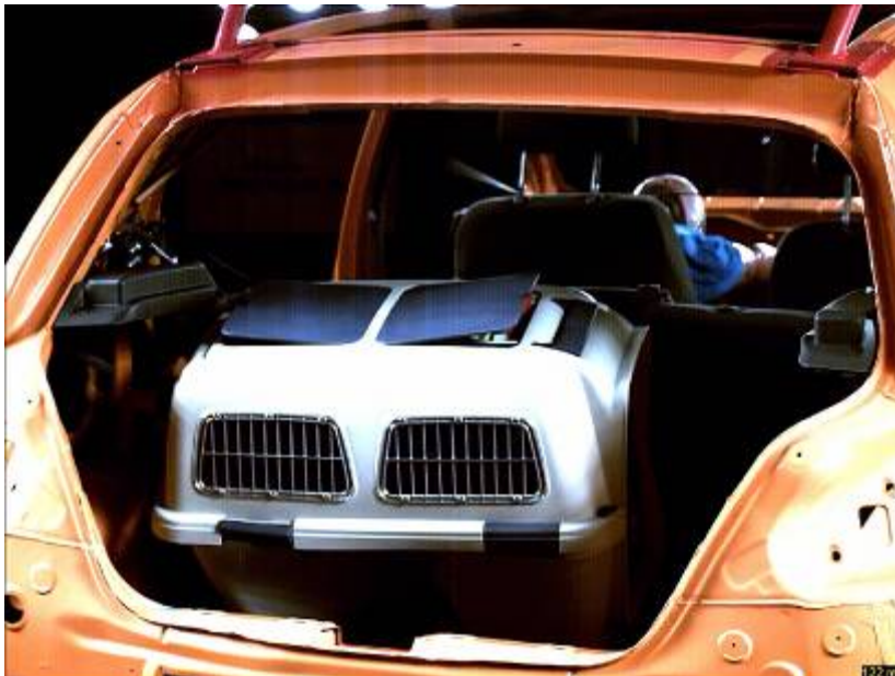
Figure 24: 125ms – upon impact, the dog carrier is pushed into the backrest
