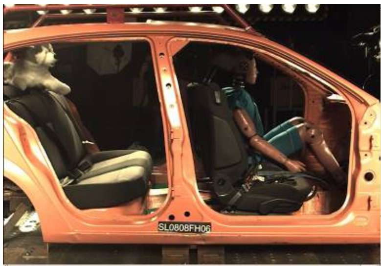
Figure 7: 0ms – the dog dummy in its original position on the car's rear window shelf
