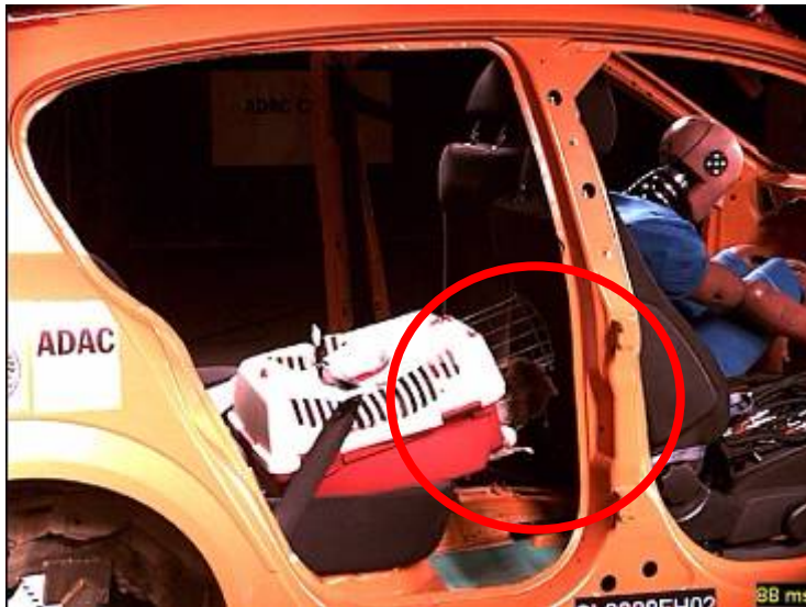
Figure 21: 90ms – the pet carrier's anchoring points burst when the cat dummy forces the trap door open
