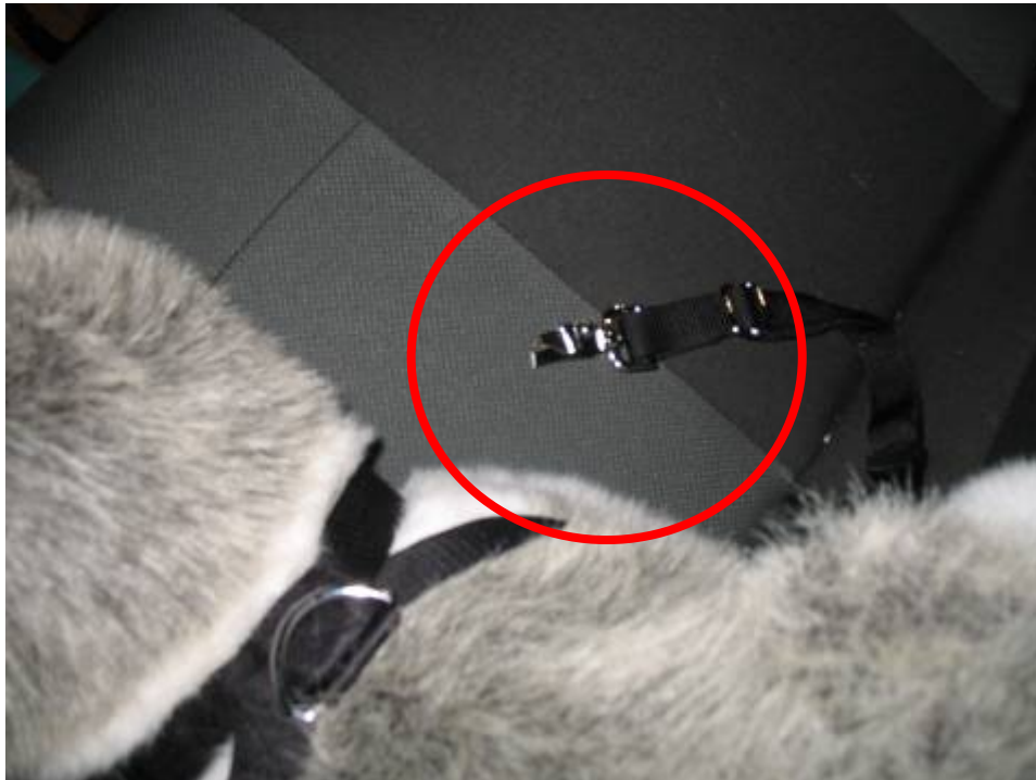
Figure 10: Broken carabiner hook
