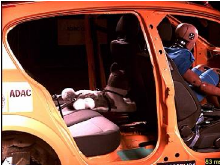
Figure 12: 83ms – with the dog dummy moving forward, the carabiner does not withstand the load and breaks
